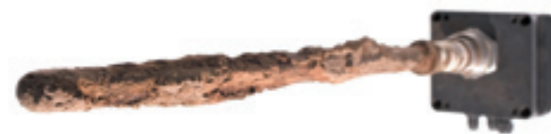
Sensor element unaffected by contamination
